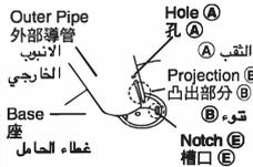
② Set the projection (B) to the notch (E) and insert outer pipe into base until hole (A) fully inserted.
