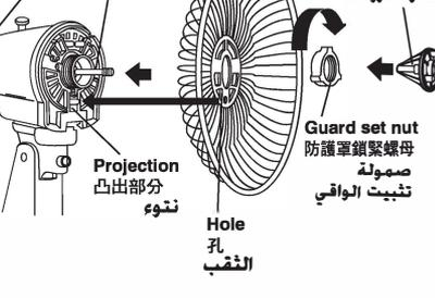
① Set the Blade Boss projection on to the Shaft Pin.
